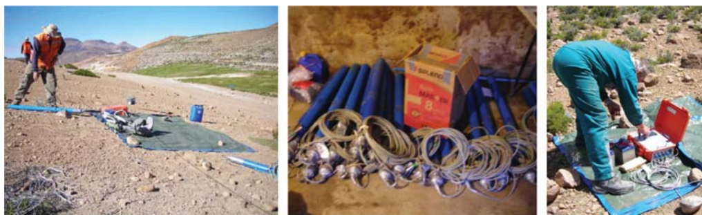
Figure 4.26. Left: preparing coils (blue tubes) for an MT station. Middle: MT coils. Right: acquisition unit at an MT station.
